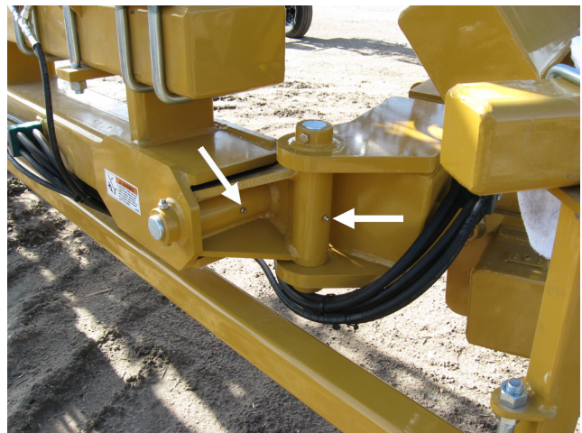
Figure 38. Wing Pivot Grease Locations
