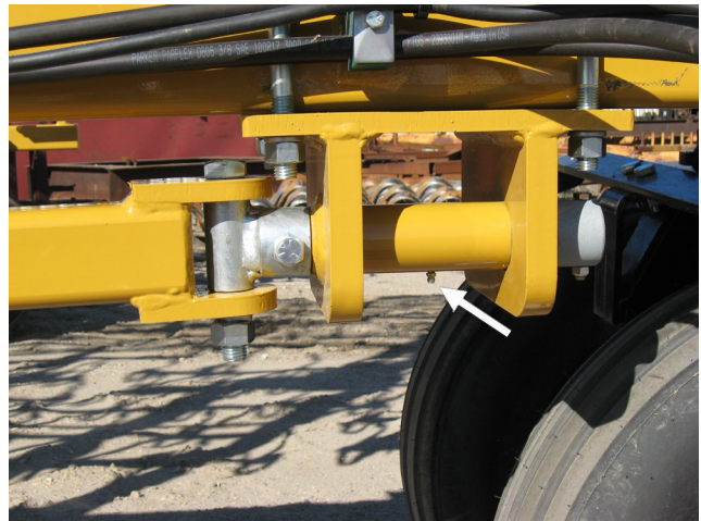
Figure 36. Wing Support Pivot Grease Location
