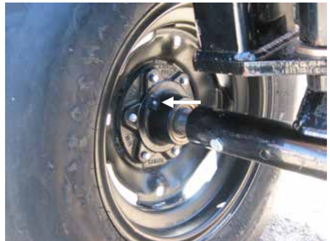
Figure 35. 5-Bolt Hub Grease Location
