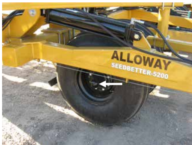
Figure 37. Main Strut Bearing Grease Location
