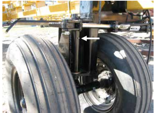
Figure 33. Wing Strut Pivot Grease Location
