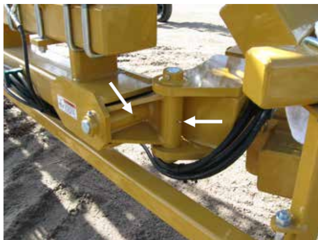
Figure 38. Wing Pivot Grease Locations
