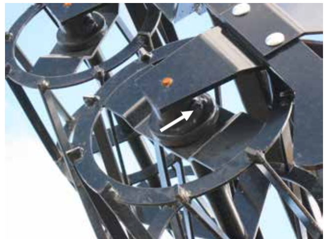
Figure 31. Crumbler Basket Grease Location
