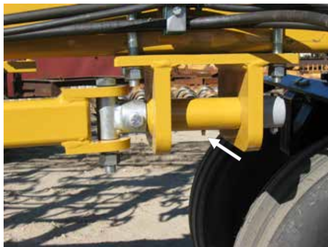
Figure 36. Wing Support Pivot Grease Location
