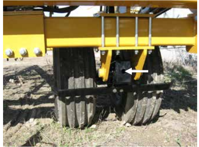
Figure 32. Main Strut Pivot Grease Location
