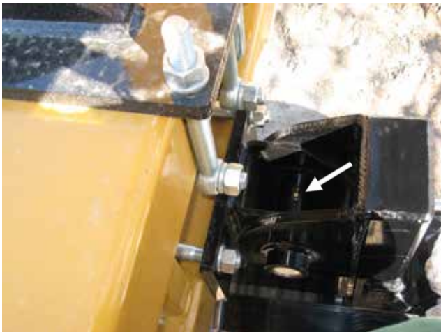
Figure 34. Wing Strut Hinge Grease Location
