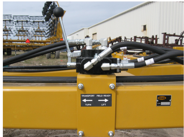
Figure 11. Valve in Transport Position
