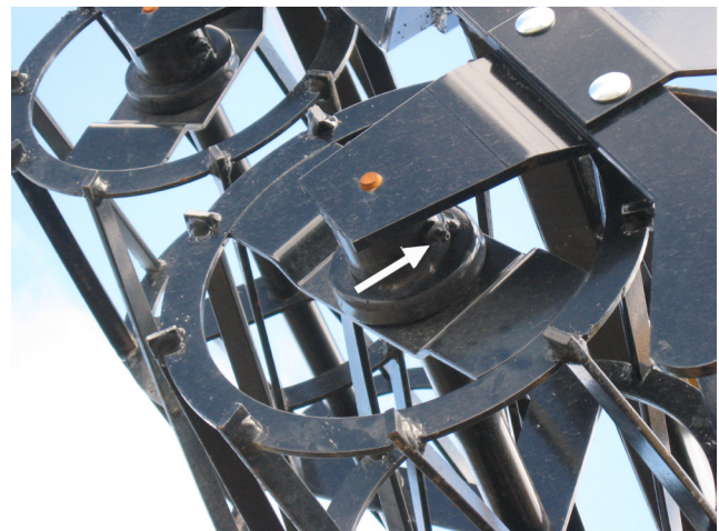
Figure 31. Crumbler Basket Grease Location
