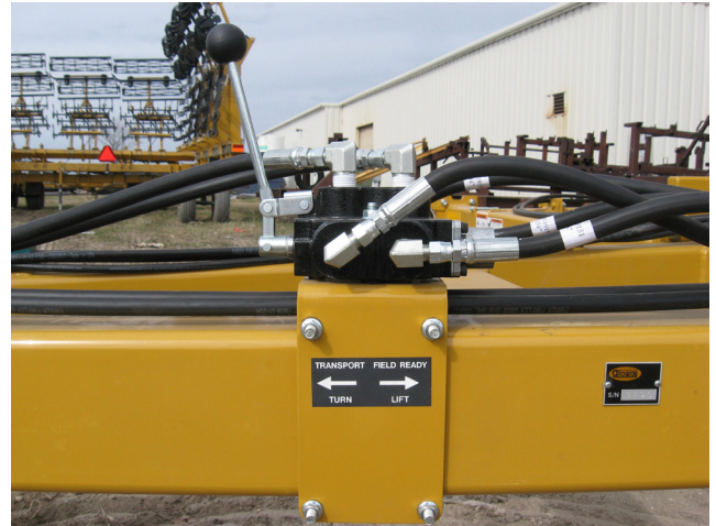
Figure 6. Valve in Transport Position
