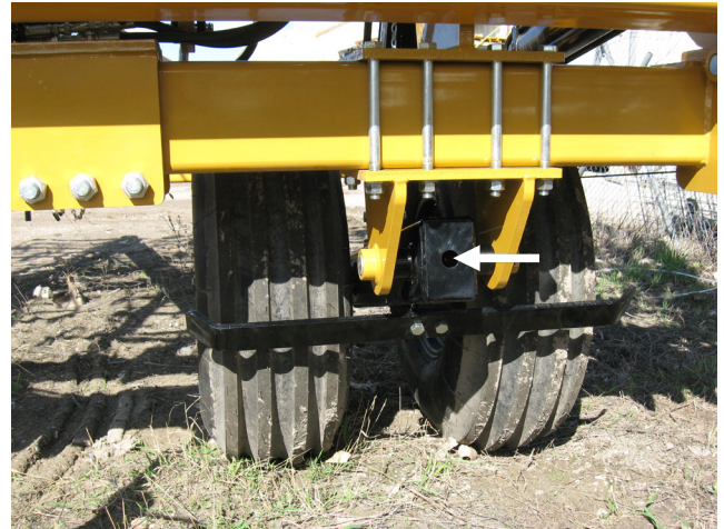
Figure 32. Main Strut Pivot Grease Location
