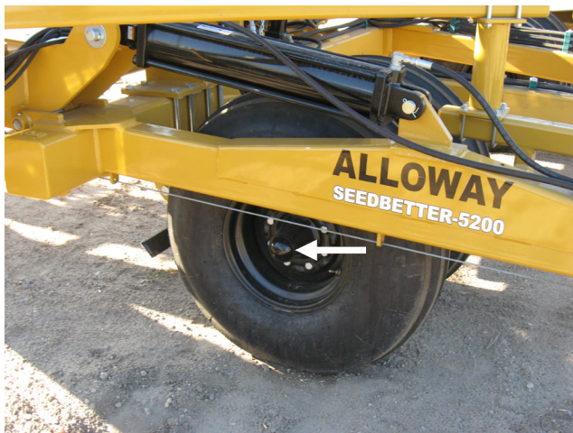
Figure 37. Main Strut Bearing Grease Location
