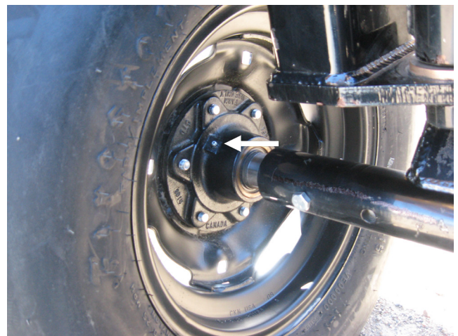
Figure 35. 5-Bolt Hub Grease Location
