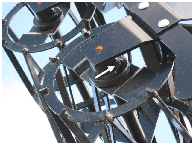
Figure 31. Crumbler Basket Grease Location
