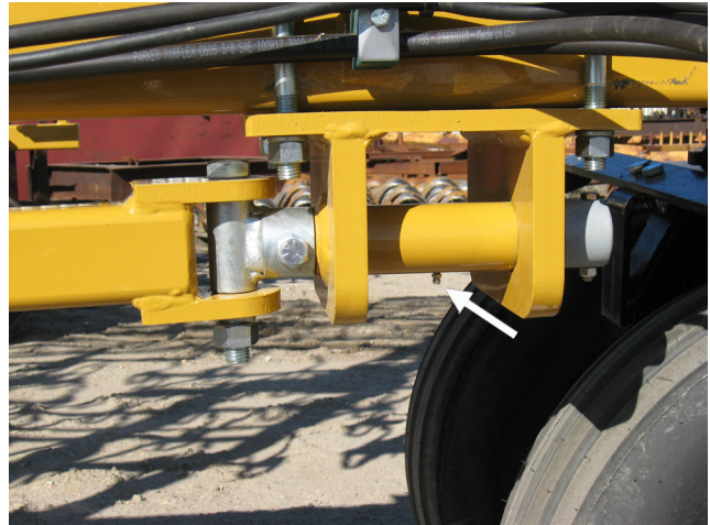
Figure 36. Wing Support Pivot Grease Location
