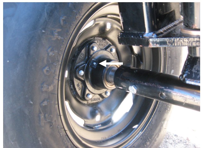
Figure 35. 5-Bolt Hub Grease Location
