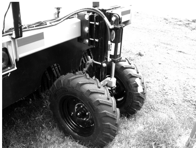
Figure 11. Wheel Mounting Bolts
