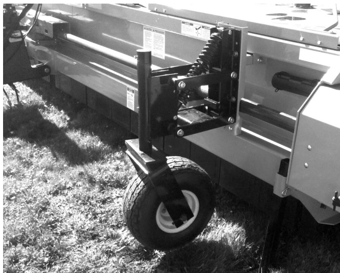
Figure 12b. Stabilizer Wheel Mounting Position
