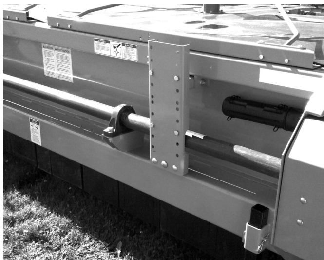
Figure 12a. Stabilizer Wheel Mount Plate
