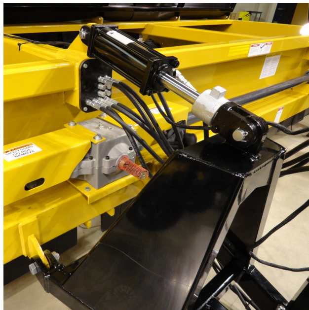
Figure 2b. PTO Driveline
