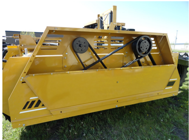
Figure 34. Rotor Upper Drive Pulleys
