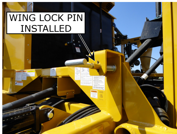
Figure 17a. Wing Lock Pin Installed
