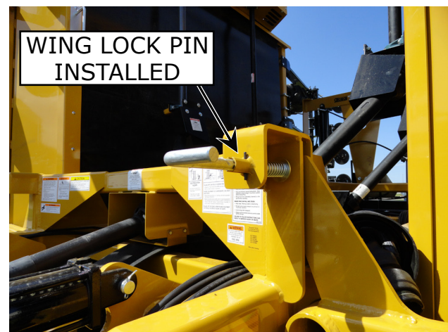
Figure 17a. Wing Lock Pin Installed
