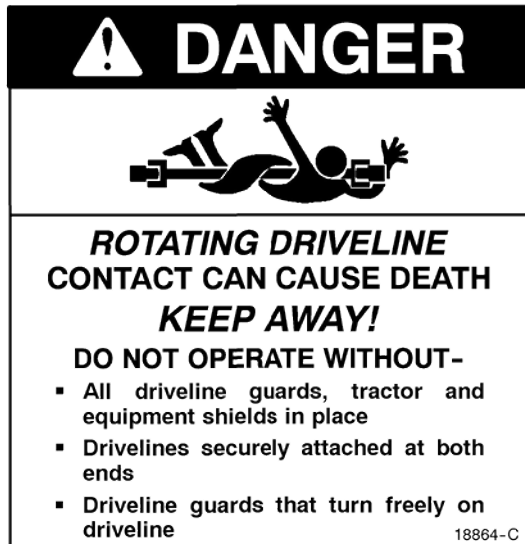
9. 506-3-0196 Rotating Driveline Warning
