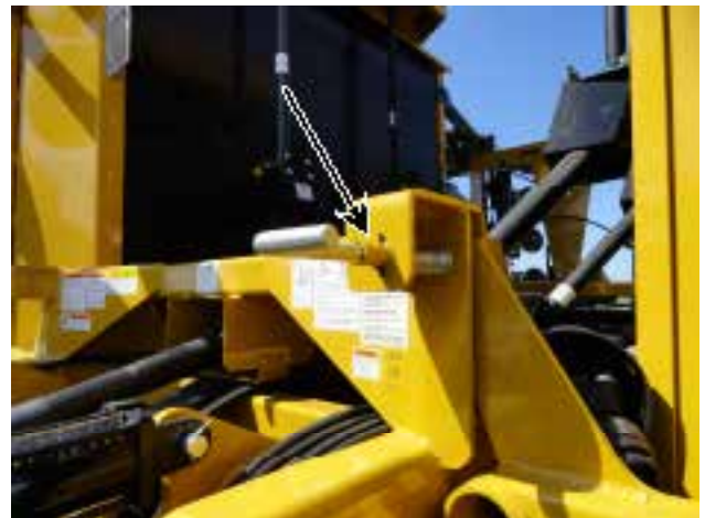
Figure 17a. Wing Lock Pin Installed
