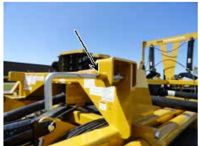
Figure 17b. Wing Lock Pin Storage
