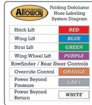
Figure 9. Hose Labeling Diagram
