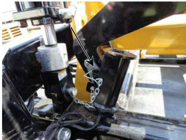
Figure 20. Rear Wheel/Lift Cylinder Lock Storage
