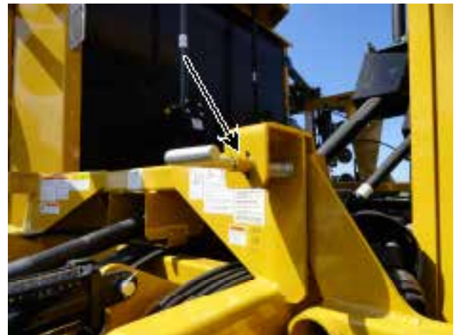
Figure 17a. Wing Lock Pin Installed
