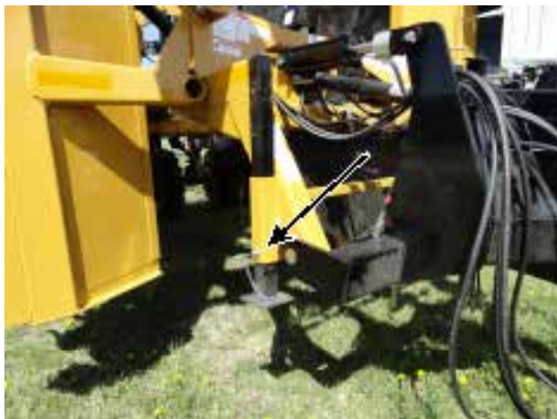
Figure 8. Parking Stand in Raised Position
