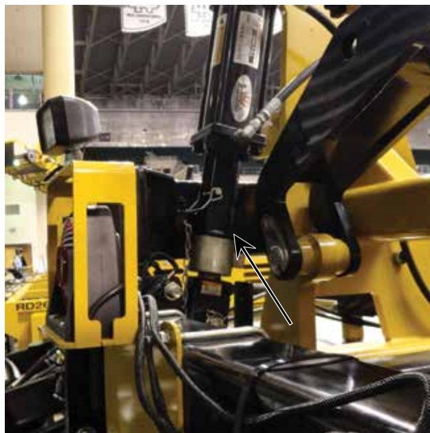
Figure 14. Rear Wheel/Lift Cylinder Lock
