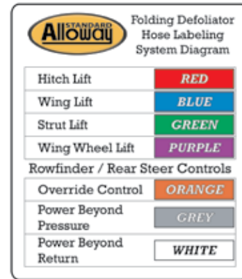
Figure 9. Hose Labeling Diagram
