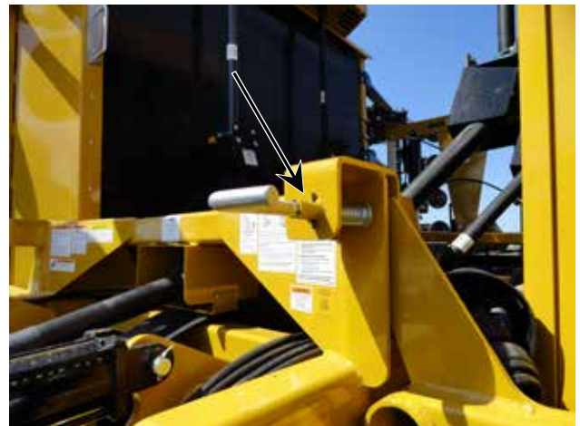
Figure 17a. Wing Lock Pin Installed
