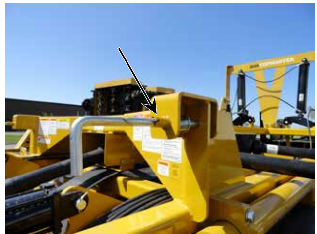
Figure 17b. Wing Lock Pin Storage
