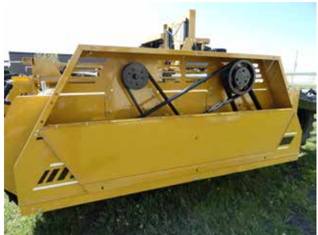
Figure 34. Rotor Upper Drive Pulleys
