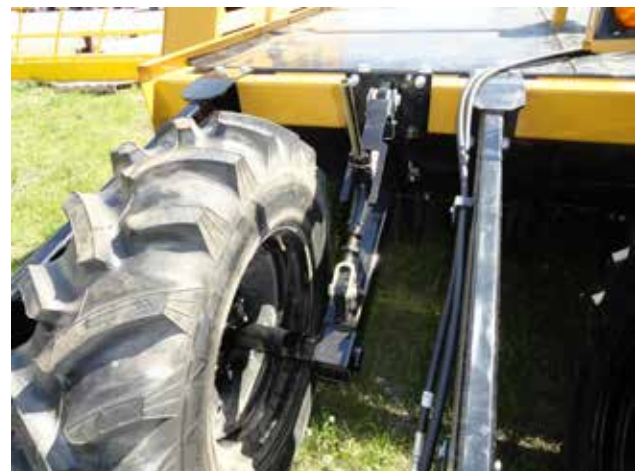
Figure 23. Gauge Wheel Ratchet Jack
