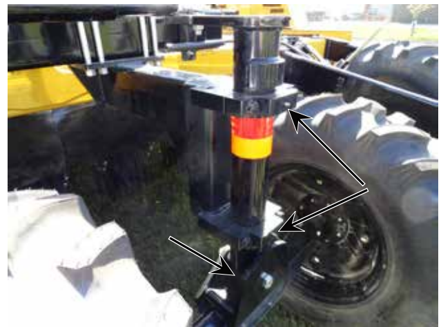
Figure 31. Rear Steering Pivots
