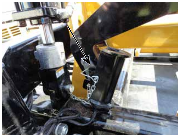
Figure 20. Rear Wheel/Lift Cylinder Lock Storage
