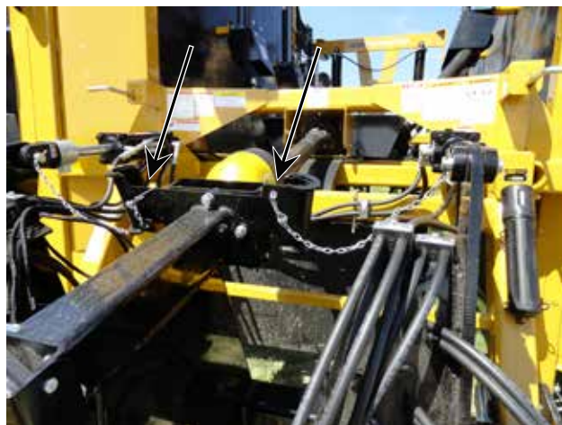
Figure 15. Front Hitch/Lift Cylinder Lock Storage
