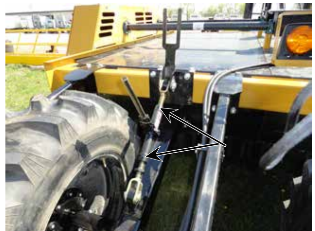
Figure 32. Gauge Wheel Jack Screws
