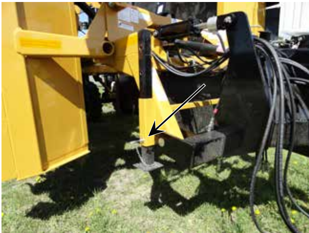
Figure 8. Parking Stand in Raised Position
