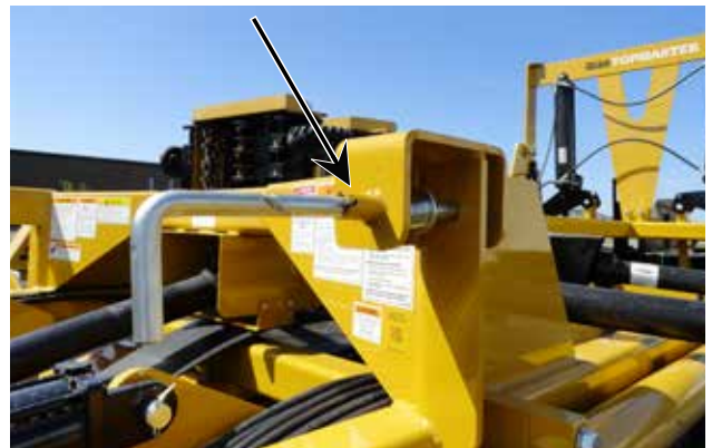
Figure 17a. Lock Pin Operate (Lowered) Position
