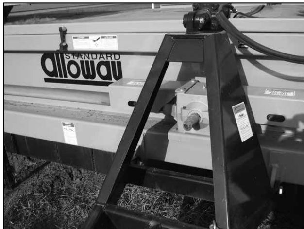
Figure 2b. PTO Driveline
