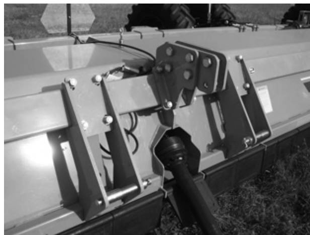
Figure 3. 3-Point Hitch Attachment
