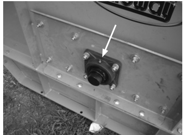
Figure 32. Rotor End Bearing Lubrication Point
