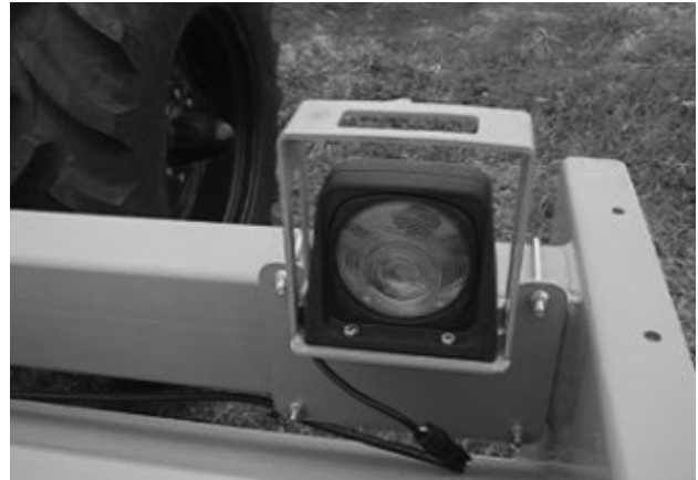
Figure 58. Safety Light Kit Installed
