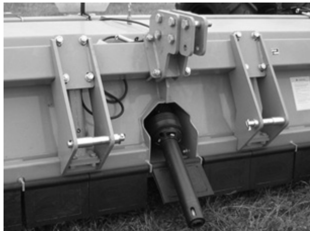
Figure 7. Attaching to 3-point model
