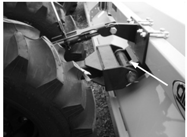
Figure 33. Wheel Strut Pivot Bearing Lubrication Points
