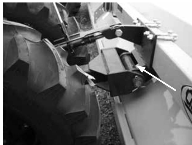
Figure 33. Wheel Strut Pivot Bearing Lubrication Points
