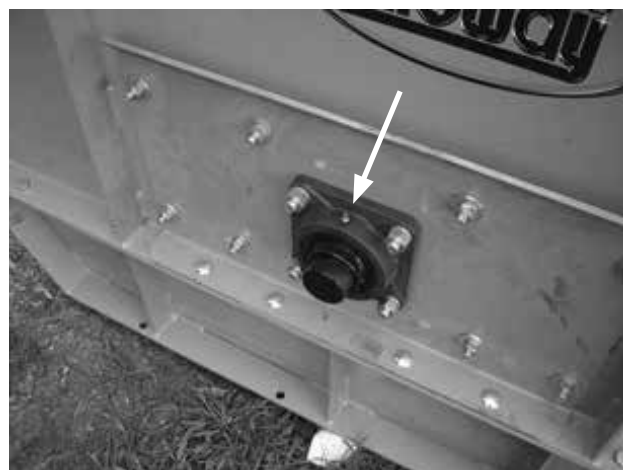
Figure 32. Rotor End Bearing Lubrication Point
