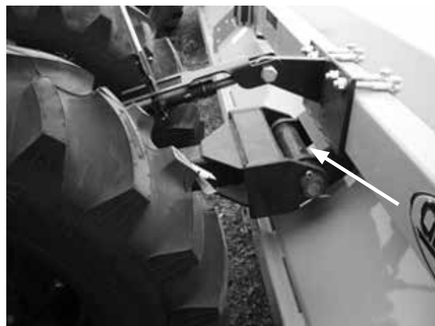
Figure 33. Wheel Strut Pivot Bearing Lubrication Points
