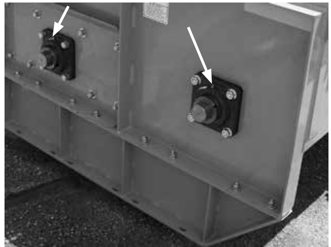
Figure 32. Rotor End Bearing Lubrication Point
