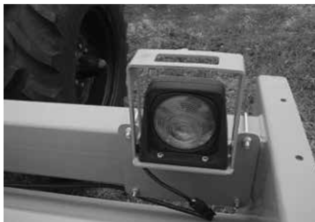
Figure 58. Safety Light Kit Installed
