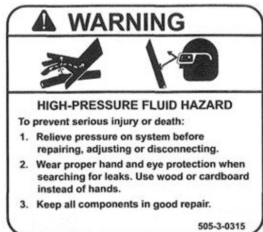
12. 505-3-0315 High Pressure Fluid Hazard Warning
