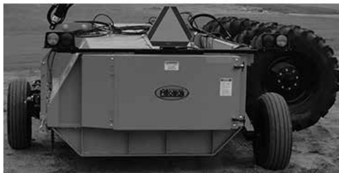
Figure 61. Dual Safety Light Kit Installed
