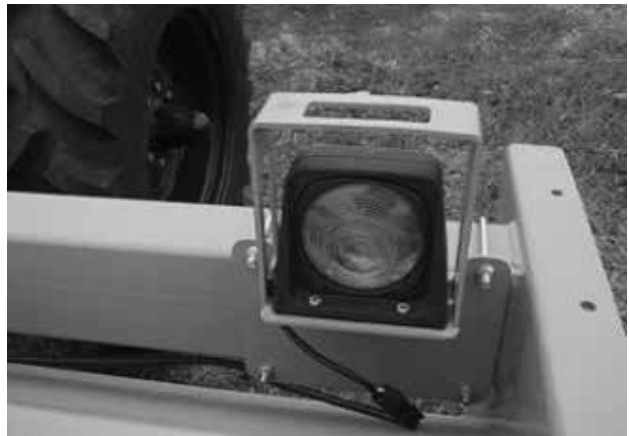
Figure 58. Safety Light Kit Installed
