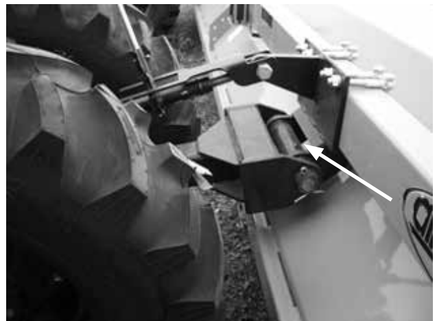
Figure 33. Wheel Strut Pivot Bearing Lubrication Points
