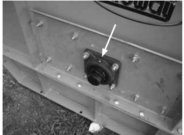
Figure 32. Rotor End Bearing Lubrication Point
