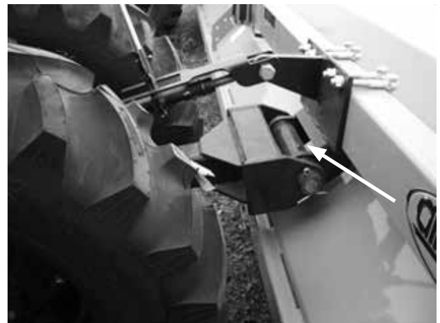
Figure 33. Wheel Strut Pivot Bearing Lubrication Points
