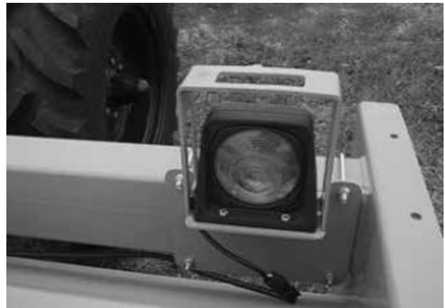
Figure 58. Safety Light Kit Installed
