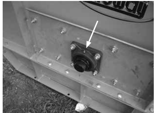
Figure 32. Rotor End Bearing Lubrication Point
