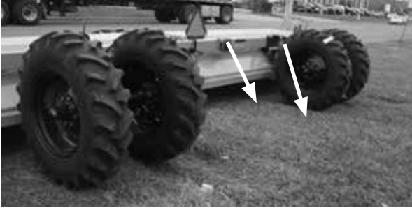
Figure 51. Wheel Assembly Installed
