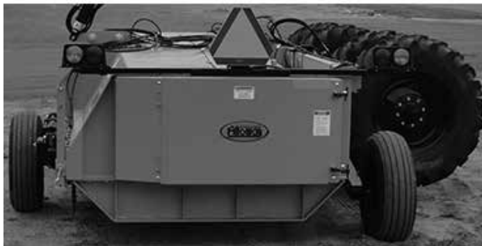
Figure 61. Dual Safety Light Kit Installed
