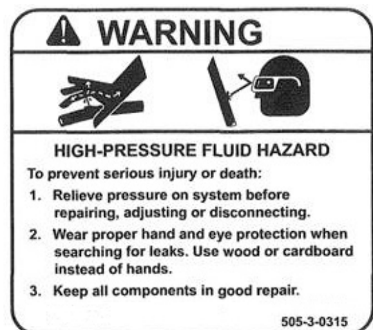
12. 505-3-0315 High Pressure Fluid Hazard Warning
