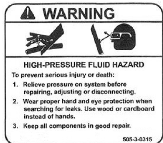
12. 505-3-0315 High Pressure Fluid Hazard Warning
