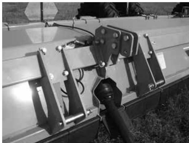
Figure 3. 3-Point Hitch Attachment
