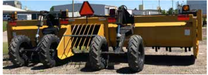
Figure 51. Wheel Assembly Installed
