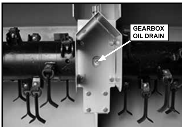
Figure 38. Drain Plug (underside of unit)
