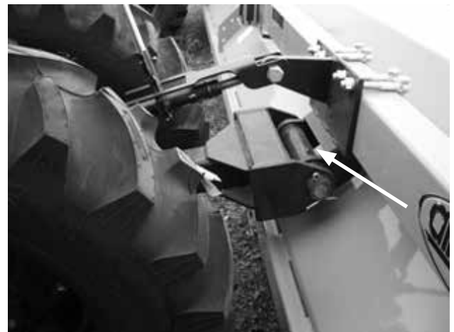
Figure 33. Wheel Strut Pivot Bearing Lubrication Points
