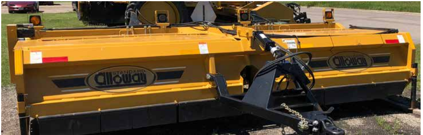
Figure 58. Safety Light Kit Installed
