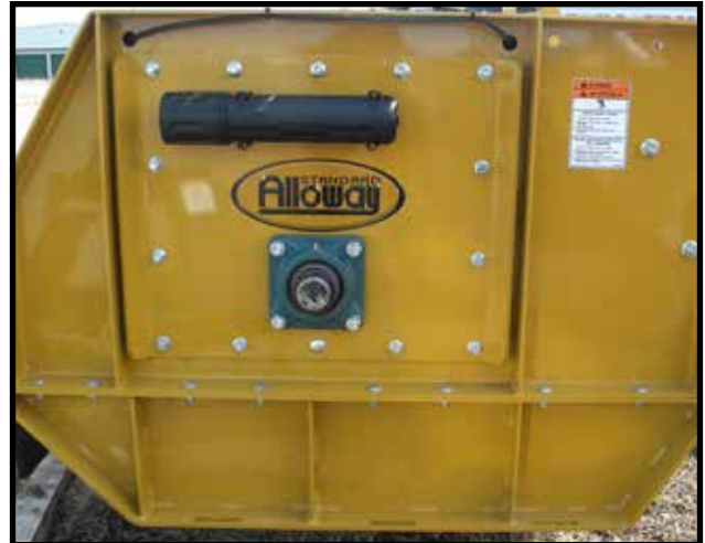
Figure 55. Manual Storage Tube Assembly
