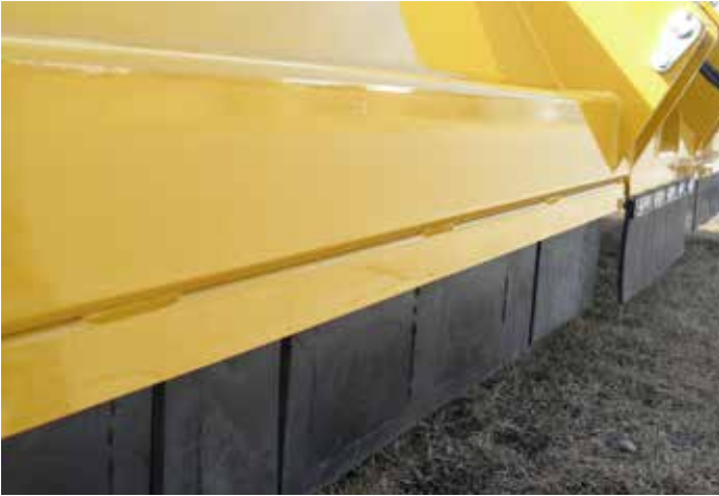
Figure 42. Front Rubber Shield Flaps
