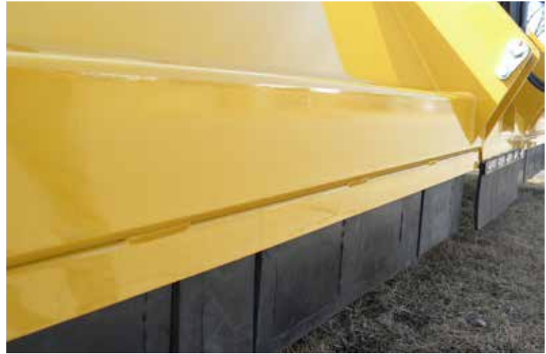
Figure 28. Front Shield Flap
