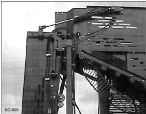
**Figure 16.** Truck Boom in Lowered Transport Position
