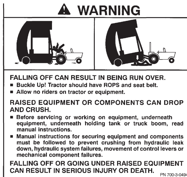
5. 700-3-0494 Fall Hazard Warning
