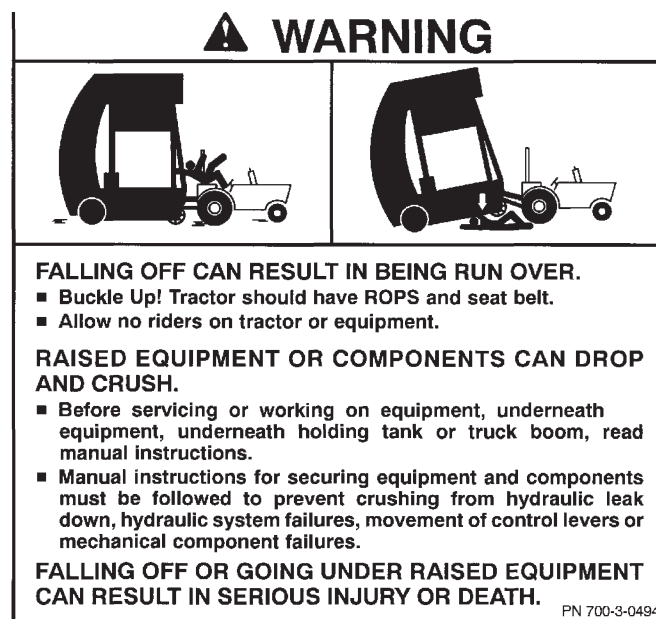
5. 700-3-0494 Fall Hazard Warning
