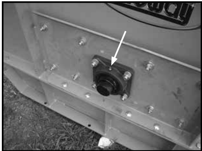
Figure 32. Rotor End Bearing Lubrication Point
