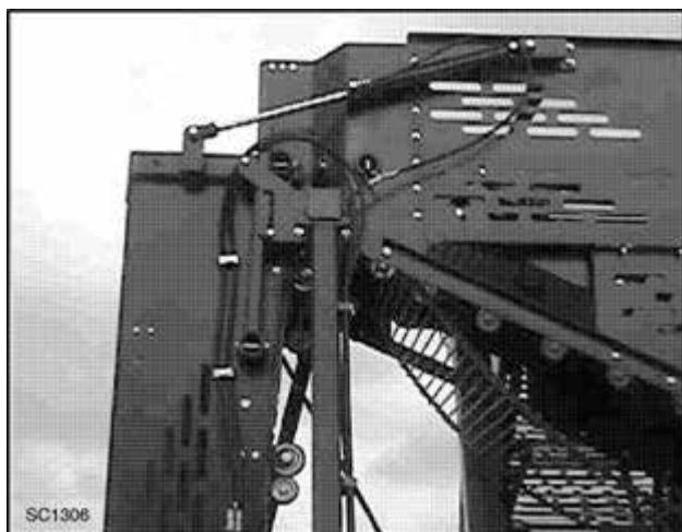
Figure 16. Truck Boom in Lowered Transport Position
