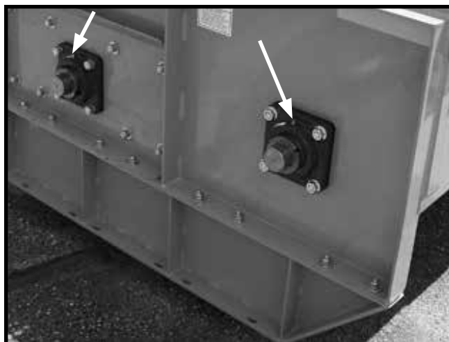
Figure 32. Auger and Rotor End Bearing Lubrication Points
