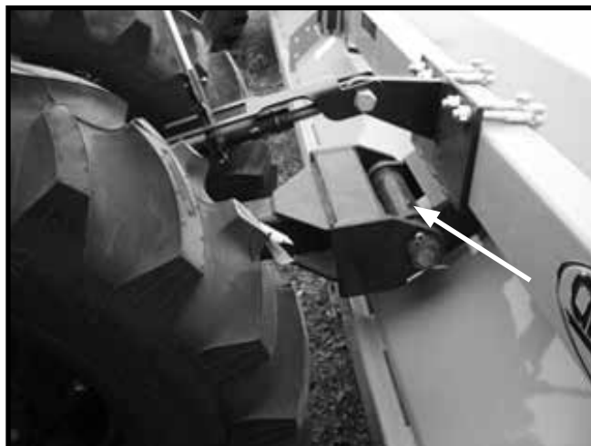
Figure 33. Wheel Strut Pivot Bearing Lubrication Points
