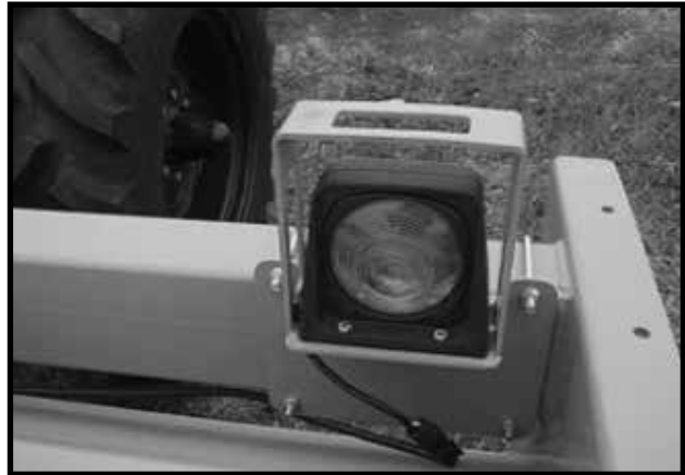
Figure 58. Safety Light Kit Installed (Non-End Tow)
