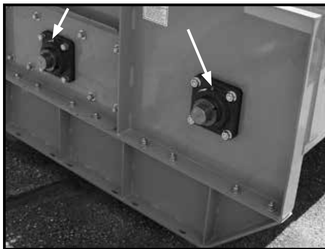
Figure 32. Auger and Rotor End Bearing Lubrication Points
