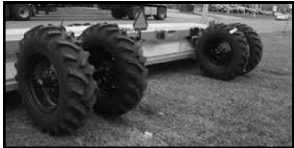
Figure 51. Wheel Assembly Installed
