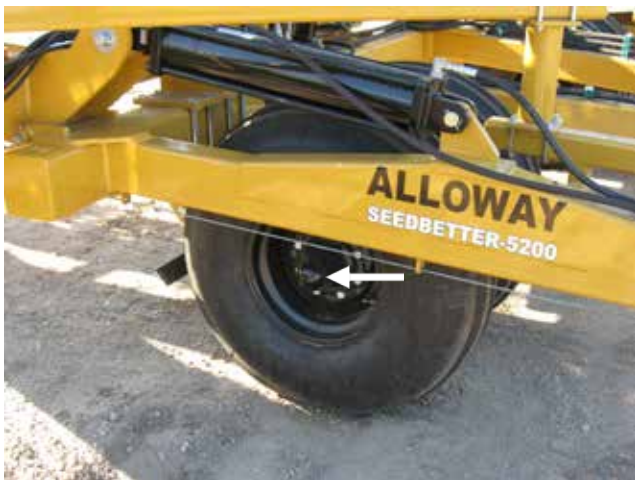
Figure 37. Main Strut Bearing Grease Location
