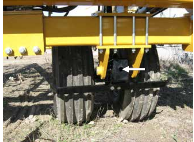
Figure 32. Main Strut Pivot Grease Location
