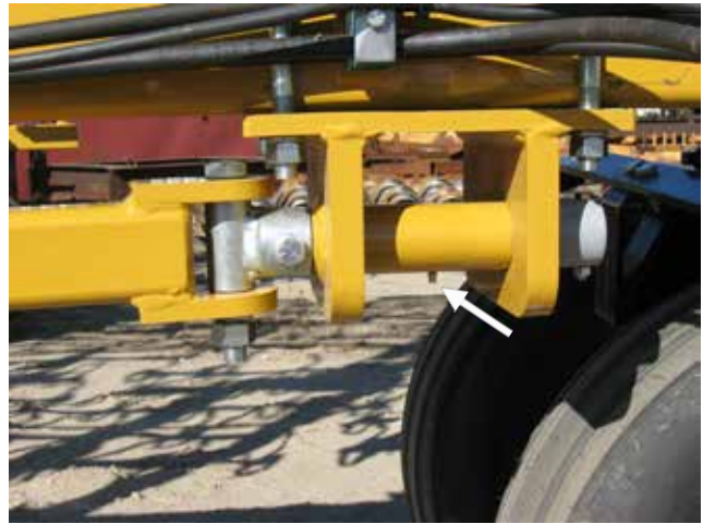
Figure 36. Wing Support Pivot Grease Location
