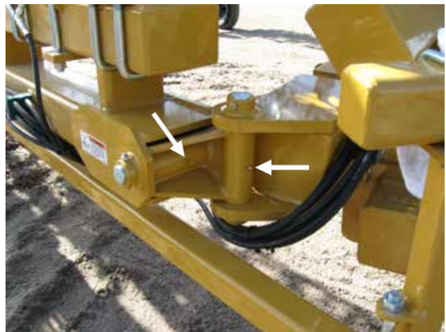
Figure 38. Wing Pivot Grease Locations
