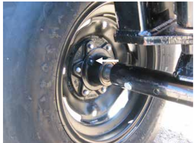
Figure 35. 5-Bolt Hub Grease Location
