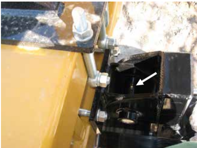
Figure 34. Wing Strut Hinge Grease Location
