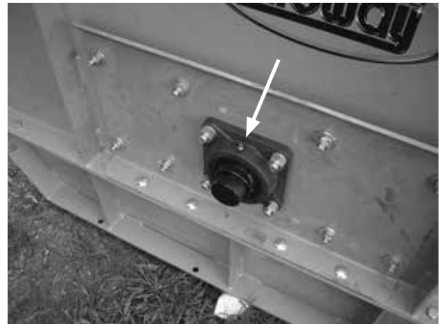
Figure 32. Rotor End Bearing Lubrication Point
