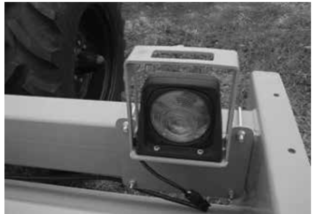
Figure 58. Safety Light Kit Installed
