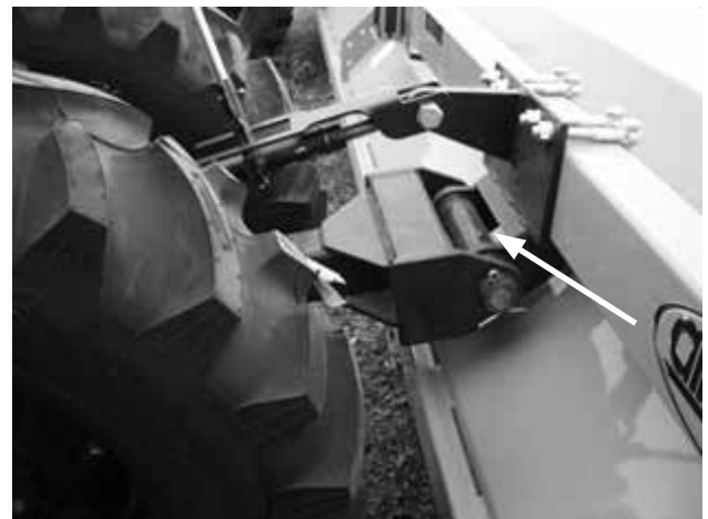
Figure 33. Wheel Strut Pivot Bearing Lubrication Points
