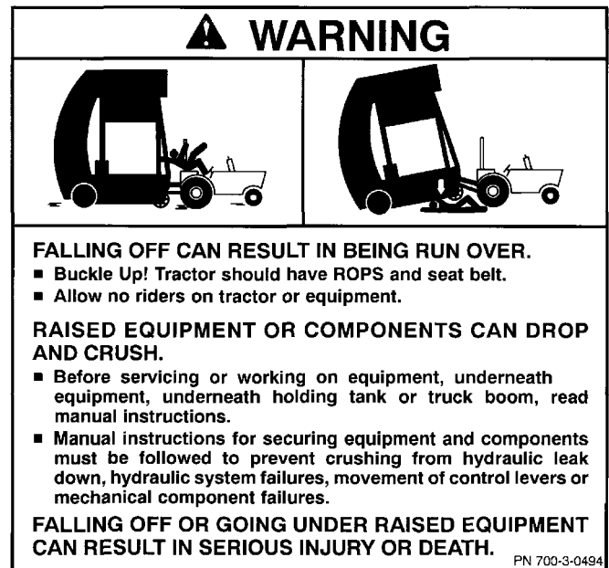
5. 700-3-0494 Fall Hazard Warning
