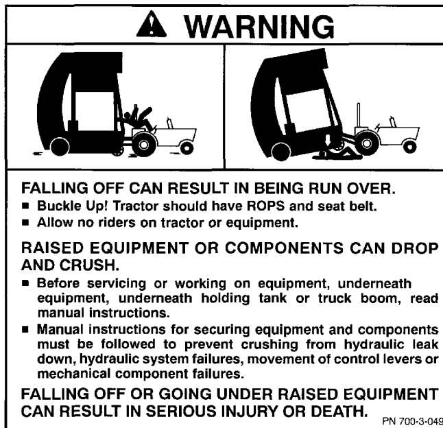
5. 700-3-0494 Fall Hazard Warning
