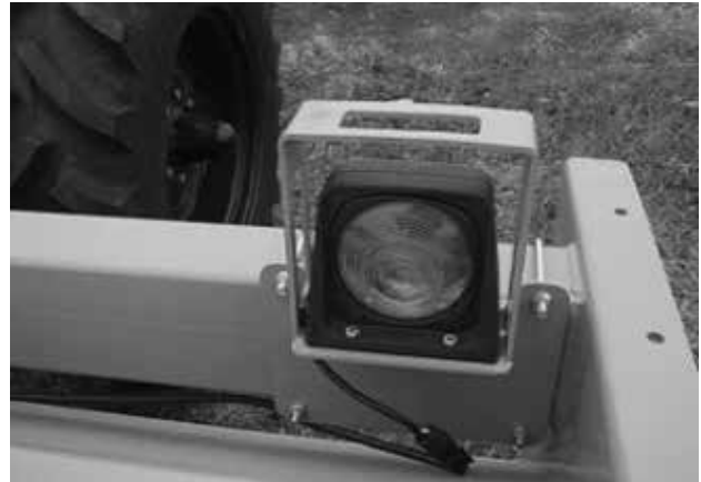
Figure 58. Safety Light Kit Installed
