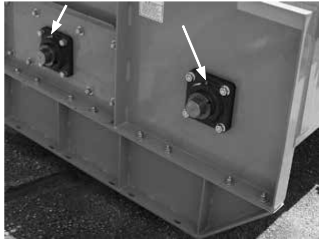
Figure 32. Rotor End Bearing Lubrication Point
