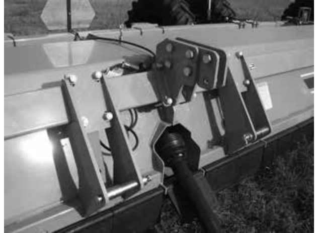
Figure 3. 3-Point Hitch Attachment
