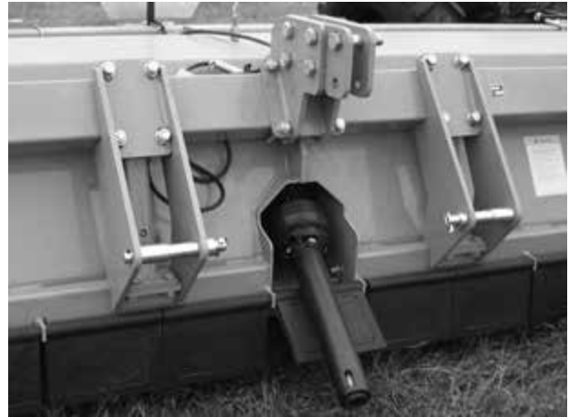
Figure 7. Attaching to 3-point model
