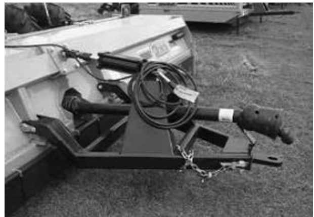
Figure 8. Attaching to Pull-type model
