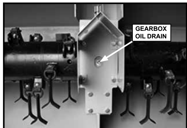
Figure 38. Drain Plug (underside of unit)
