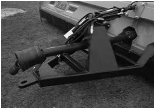
Figure 54. Pull-type Hitch Installed
