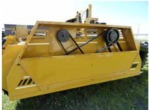
Figure 34. Rotor Upper Drive Pulleys
