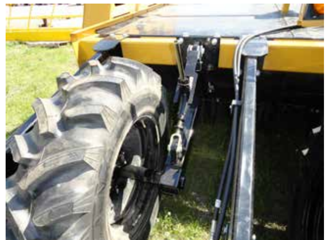
Figure 23. Gauge Wheel Ratchet Jack
