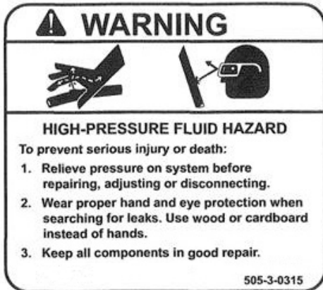
22. 505-3-0315 High - Pressure Fluid Hazard
