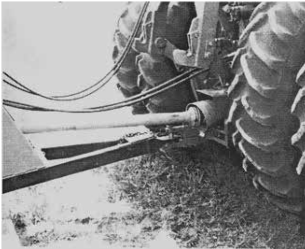
Figure 3. Driveline and Hydraulics Attached
