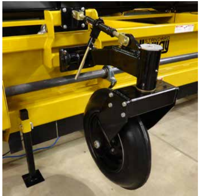
Figure 12a. Stabilizer Wheel Mounting Position
