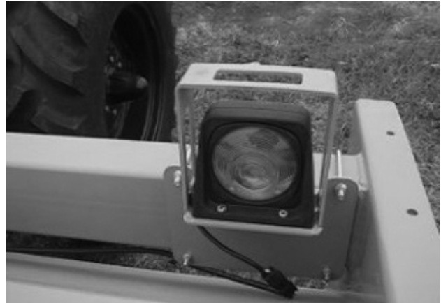
Figure 58. Safety Light Kit Installed
