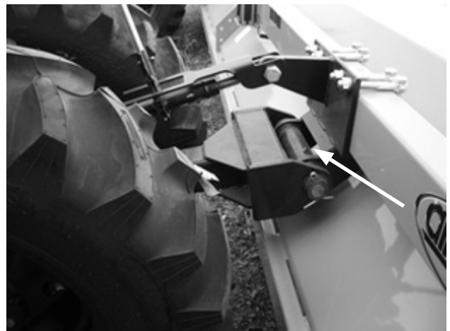
Figure 33. Wheel Strut Pivot Bearing Lubrication Points
