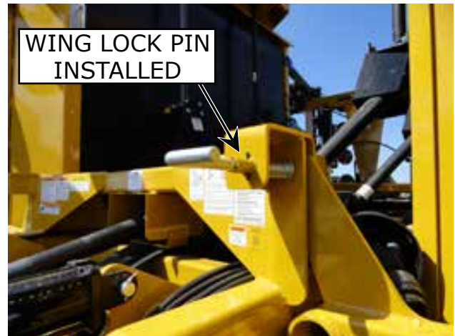
Figure 17a. Wing Lock Pin Installed
