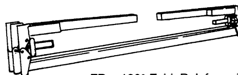
FR = 180° Fold Reinforced Double Bar
