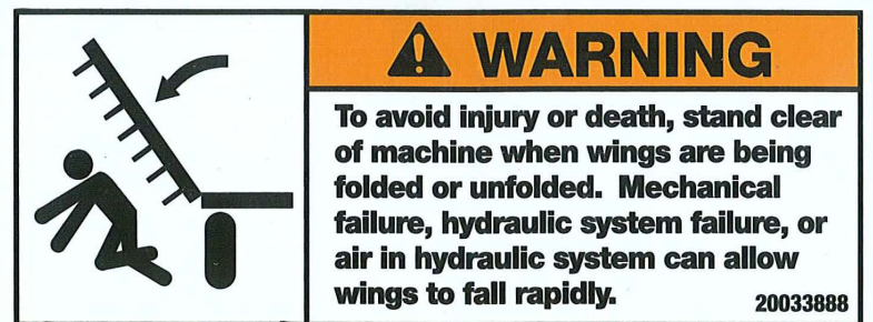
M. 200-3-3888 Raised Wing Hazard
