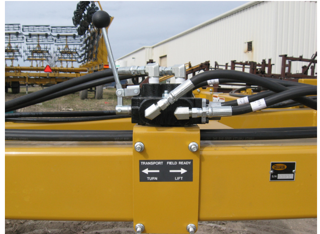
Figure 6. Valve in Transport Position
