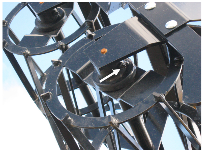
Figure 31. Crumbler Basket Grease Location
