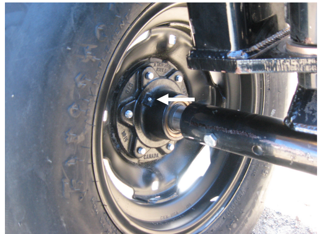
Figure 35. 5-Bolt Hub Grease Location
