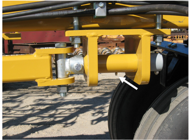
Figure 36. Wing Support Pivot Grease Location
