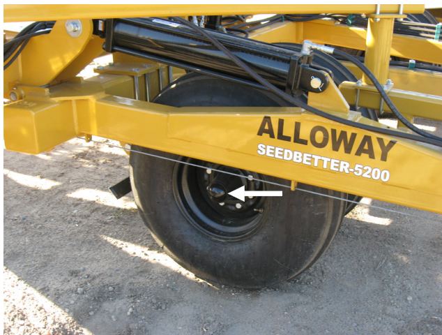
Figure 37. Main Strut Bearing Grease Location
