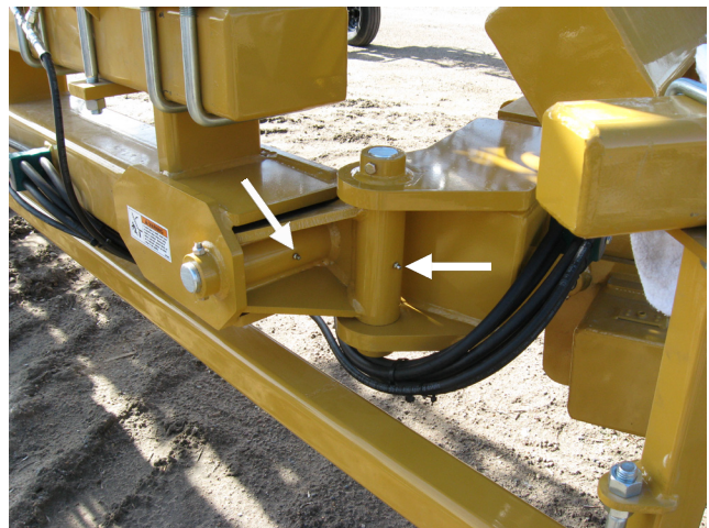
Figure 38. Wing Pivot Grease Locations
