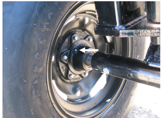
Figure 35. 5-Bolt Hub Grease Location
