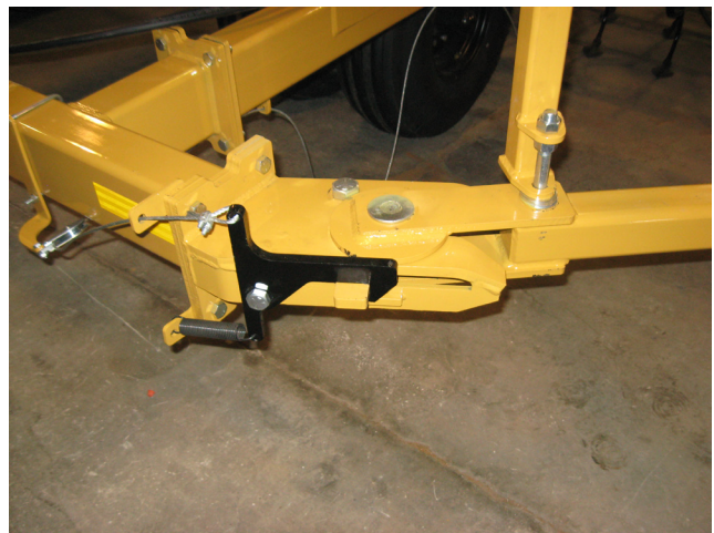
Figure 9. Pin in Locked Position
