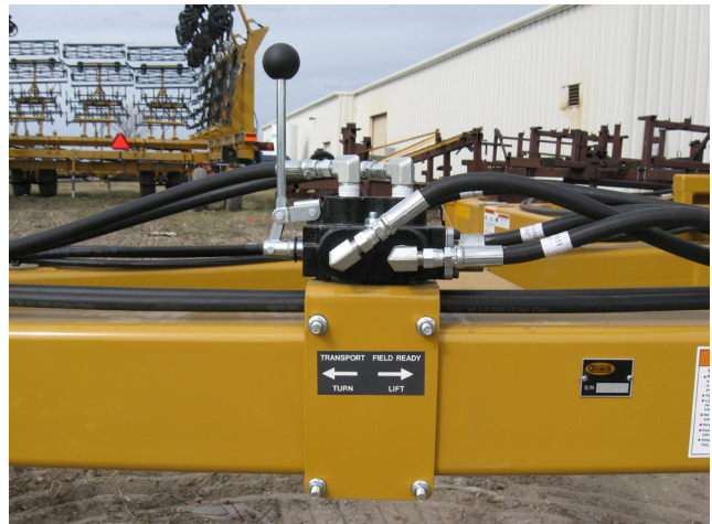
Figure 10. Valve in Field Ready Position
