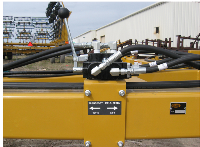
Figure 11. Valve in Transport Position
