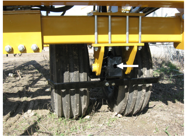
Figure 32. Main Strut Pivot Grease Location
