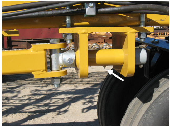
Figure 36. Wing Support Pivot Grease Location
