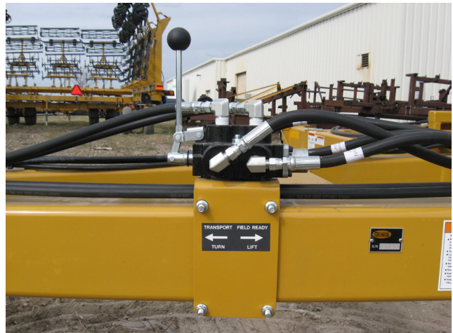
Figure 10. Valve in Field Ready Position
