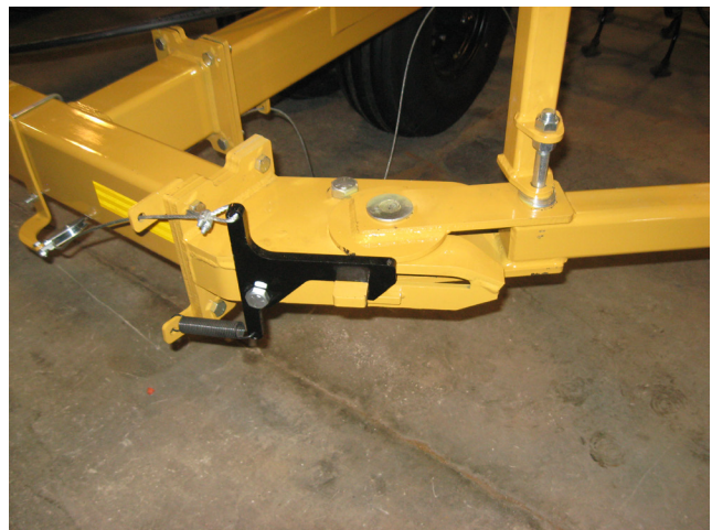
Figure 9. Pin in Locked Position
