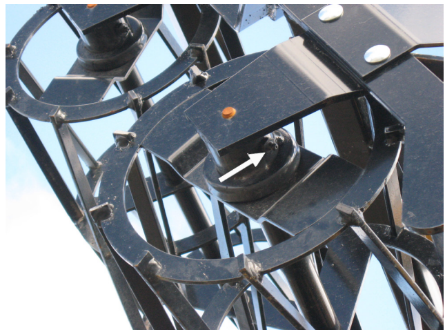
Figure 31. Crumbler Basket Grease Location
