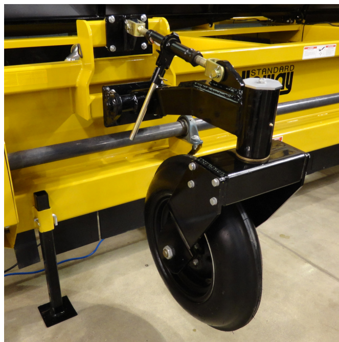
Figure 12a. Stabilizer Wheel Mounting Position
