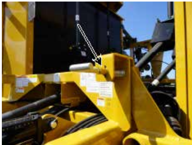
Figure 17a. Wing Lock Pin Installed
